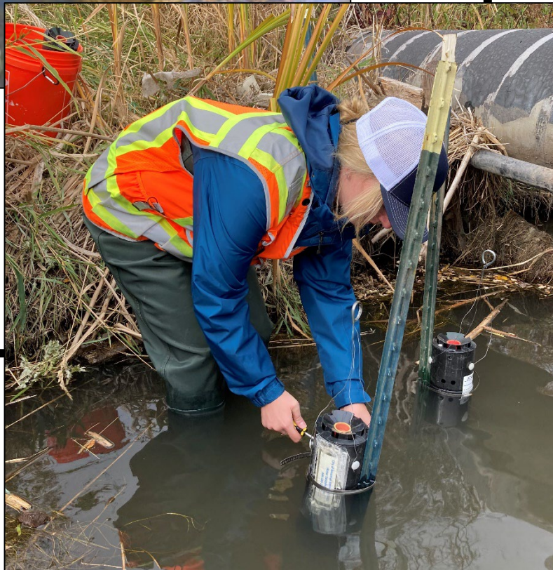
Graphic 8.0.2: Installing in-stream sampling equipment
