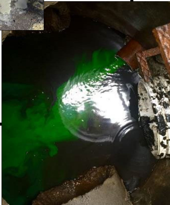
Graphic 4.0.2: Illicit connection confirmation
