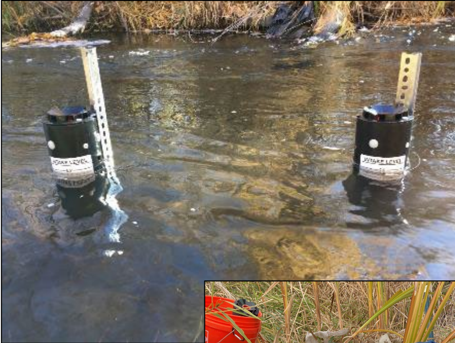
Graphic: 8.0.1: In-stream sampling equipment
