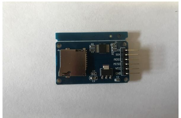
Let's start with testing the module and the SD card. Wire up the following circuit . CS->4, SCK->13,1, Mosi->11, Miso->12
