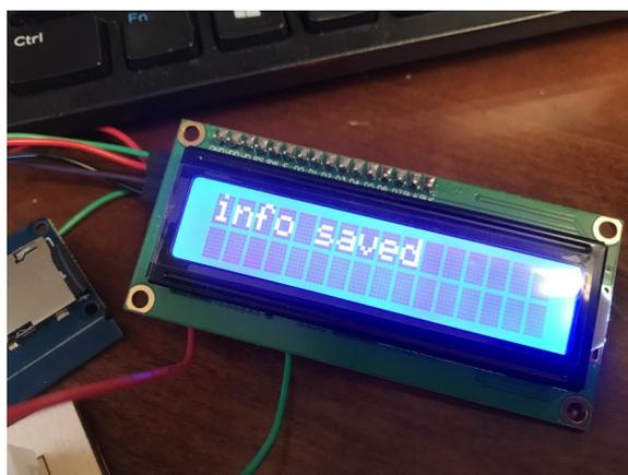
After we wait for awhile we can turn off the circuit and pull the SD card. Using a SD card we can plug in the pc and open up the drive. You should see a data log file as .txt file. We can open it and see our data.
