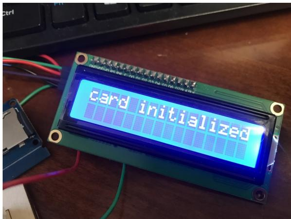
After the setup, the circuit will take a temperature reading and will display on the LCD.
