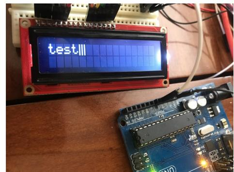
Now that we have the basic functionality of the LCD screen down, let's look at a way to simplify the wiring. We are going to use the I<sup>2</sup>C ([inter-integrated circuit](#)) adaptor for the LCD to condense the wires down to 4. To start find your I<sup>2</sup>C adaptor and attach it to your LCD. Next create the circuit below.
