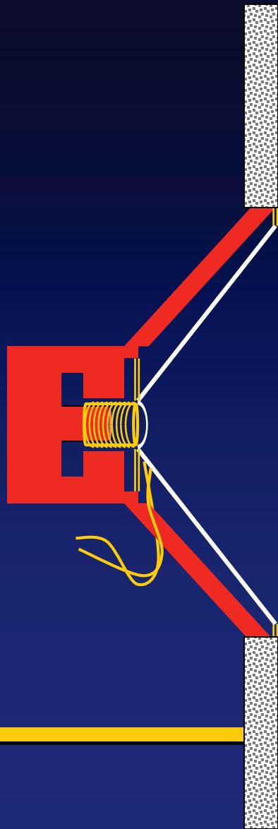
Baffle prevents front-back interaction: improved low frequency performance
