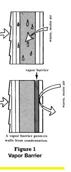
moisture. Vapor barriers should always be placed near the warm side of a wall, floor and ceiling. Materials near the cold side should let moisture escape from the wall or ceiling to the outside. A vapor barrier placed on both the warm and cold side may trap moisture causing problems.
