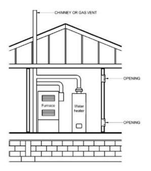
Each opening shall have a minimum <u>free area</u> of 1 square inch per 1,000 Btu/h of the total input rating of all appliances in the space, but not less than 100 square inches. (Total BTU Input of all Appliances / 1,000 = Free Area Of Each Opening Required )
