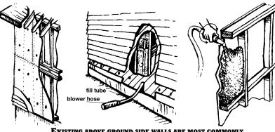
EXISTING ABOVE GROUND SIDE WALLS ARE MOST COMMONLY INSULATED BY REMOVING SIDING OR DRILLING HOLES INTO THE SIDEWALL AND BLOWING LOOSE-FILL INTO CAVITIES.
