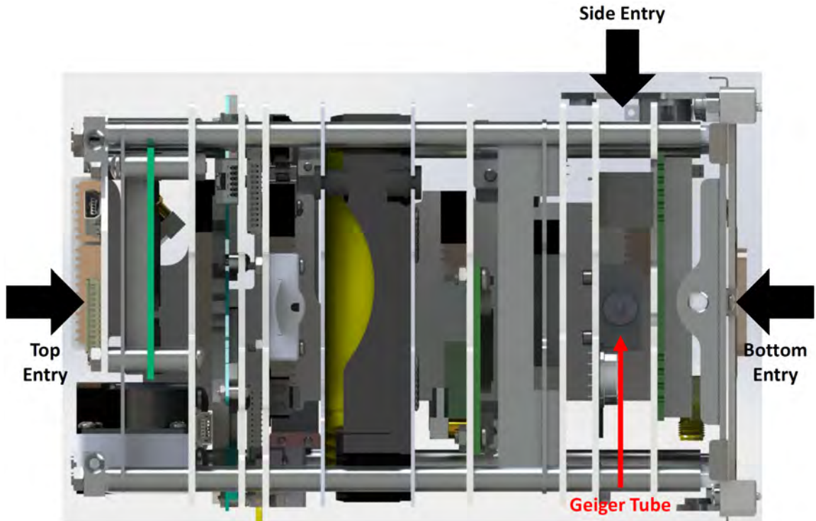
Figure 19: Cross-section of EDSN spacecraft shown without any solar panels. The three major particle entrance locations described in this analysis are shown in black.
