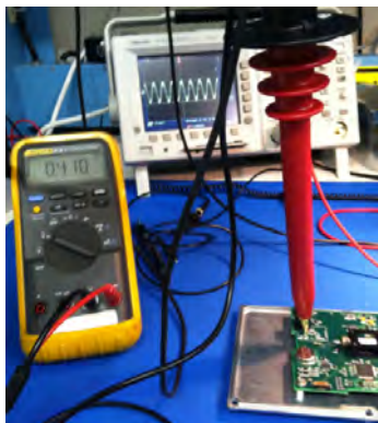
Figure 34: The 1 G \Omega probe and multimeter used to take the truth measurement in the high voltage circuit monitor calibration, meter is currently reading 410V. The oscilloscope in the background is displaying an example of the HVPS ripple voltage, measured earlier.
