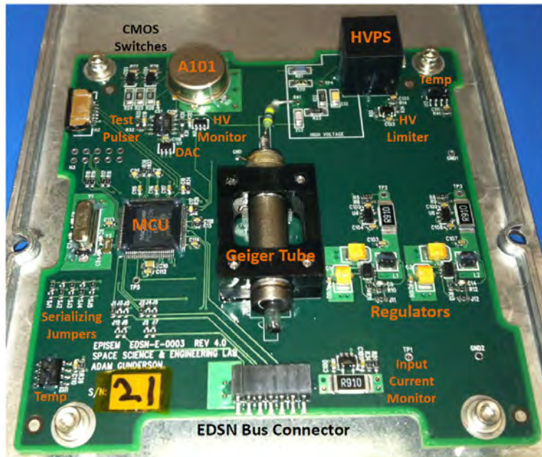
Figure 14: Image of the EPISEM circuit board displaying the location of the primary circuits and components.
