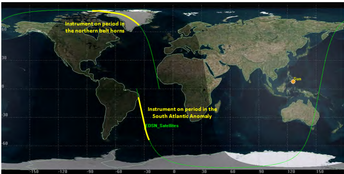
Figure 52: The ten minute periods (shown in yellow) that the instrument will be turned on once a day as simulated in STK
