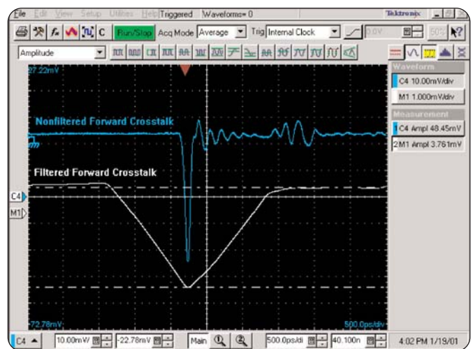
Figure 7. Forward Crosstalk Measured
