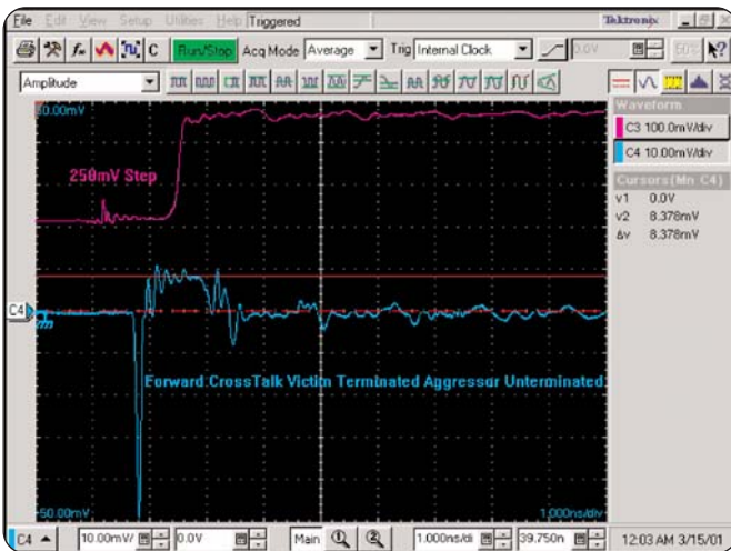
Figure 13. Measured crosstalk without end termination
