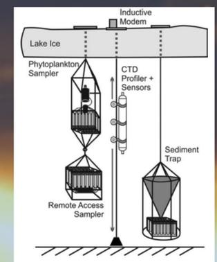
**Figure 6:** Schematic of the ice-tethered profiler (Not to scale)
