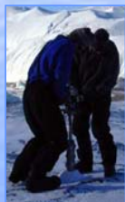
Fig. 2 Drilling ice cores with 10cm SIPRE corer
