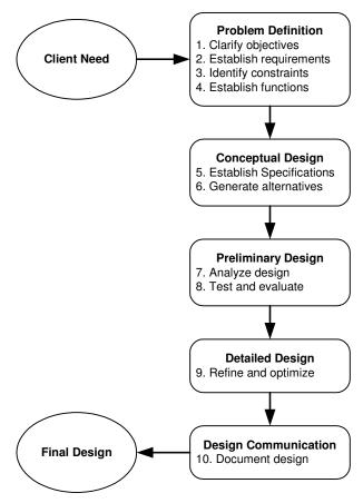
FIGURE 1: A TYPICAL DESIGN PROCESS MODEL (ADAPTED FROM DYM AND LITTLE<sup>3</sup>)
